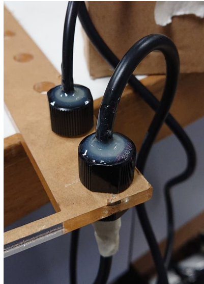
Figure 4: Hollow screw with wire fixed by epoxy
