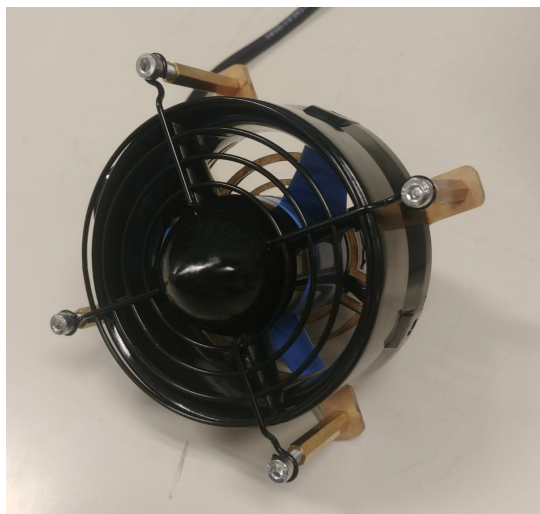
Figure 23: Thruster with safety cover
